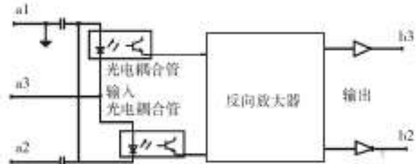
图2 回输信号处理电路 Fig. 2 Diagram of feedback signal processing circuit
