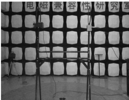
图3 环天线校准装置 Fig.3 Loop antenna calibration device
