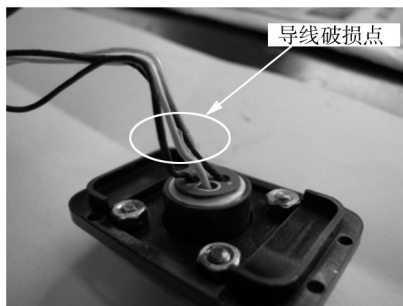
图5 导线磨损故障 Fig. 5 Wire wear failure
