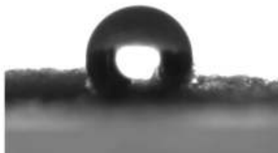
图2 SiO 2 气凝胶颗粒的接触角 Fig.2 Contact angle of SiO 2 aerogel particles
