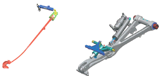
图2 F-35的A型空军型和C型海军型拦阻钩 Fig.2 Arresting hook with config A for the air force and config C for the navy of F-35
