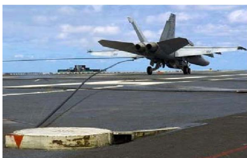
图1 舰载机典型拦阻过程 Fig.1 Typical arresting process of carrier aircraft
