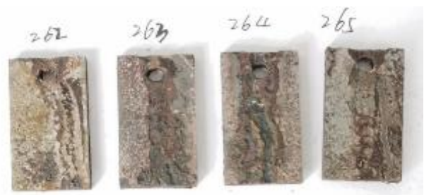
图 5 生产井井中 3Cr 管材试样腐蚀实验后 (清洗后) 表面宏观形貌 Fig.5 The surface macro morphology of 3Cr pipe samples in the middle of production well after corrosion test (after cleaning)
