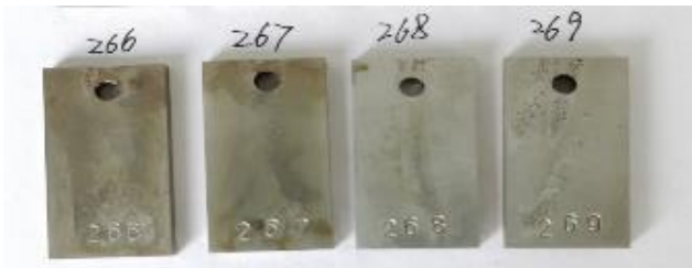
图 3 生产井井口 3Cr 管材试样腐蚀实验后 (清洗后) 表面宏观形貌 Fig.3 The surface macro morphology of 3Cr pipe samples at wellhead of production well after corrosion test (after cleaning)
