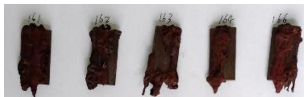
图 8 生产井井底 13Cr 管材试样腐蚀实验后表面宏观形貌 Fig.8 The surface macro morphology of 13Cr pipe samples at the bottom of production well after corrosion test
