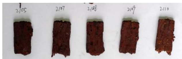
图 6 生产井井底 3Cr 管材试样腐蚀实验后表面宏观形貌 Fig.6 The surface macro morphology of 3Cr pipe samples at the bottom of production well after corrosion test
