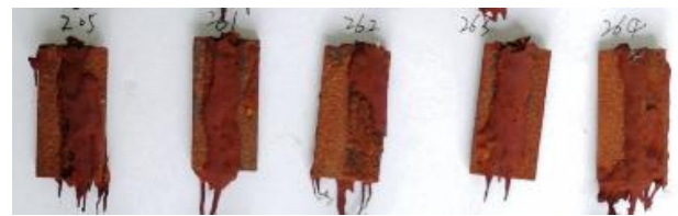
图 4 生产井井中 3Cr 管材试样腐蚀实验后表面宏观形貌 Fig.4 The surface macro morphology of 3Cr pipe samples in the middle of production well after corrosion test
