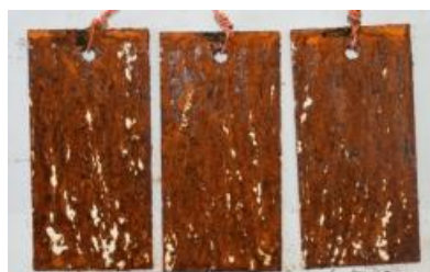
a 40CrNiMoA+镀银酸性盐雾 192 h
