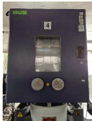
图1 温度-湿度-振动三综合试验箱 Fig.1 Temperature humidity vibration three comprehensive test chamber
