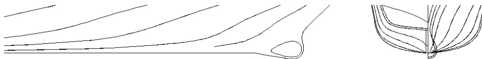
图 2 圆舭船型纵剖面图及横剖面 Fig.2 Longitudinal and cross sections of round bilge ship
