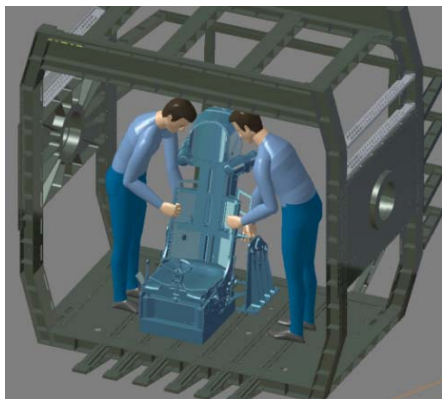
图 8 座舱座椅先于仪表台安装仿真 Fig.8 Cockpit seats are installed before the dashboard simulation
