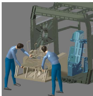
图 8 座舱座椅先于仪表台安装仿真 Fig.8 Cockpit seats are installed before the dashboard simulation
