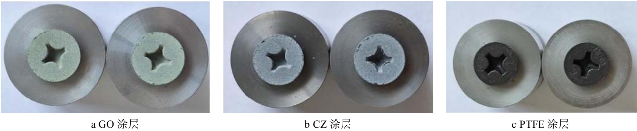
图 2 不同表面处理/涂料涂覆的钛合金紧固件 Fig.2 Titanium alloy fasteners with different surface treatments/coatings: c) GO coating; d) CZ coating; e) PTFE coating
