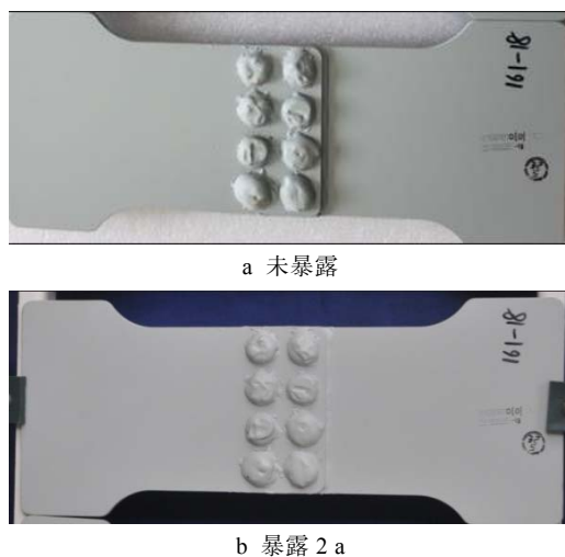
图8 典型结构件未暴露和暴露2 a后的形貌 Fig.8 Morphology of typical structural parts after 2 years of exposure: a) unexposed; b) exposed for 2 a
