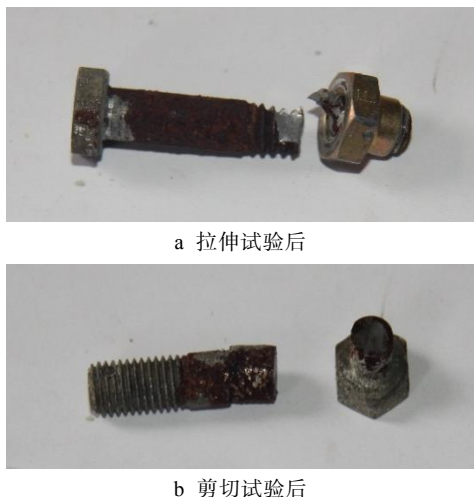
图5 经抗拉强度和剪切强度测试试验件形貌 Fig.5 Morphology after tensile strength test and shear strength test: a) after tensile strength test; b) after shear strength test
