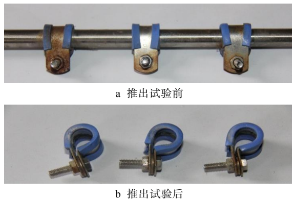
图7 推出力测试前后试验件的形貌 Fig.7 Morphology of parts before (a) and after (b) pushing force test
