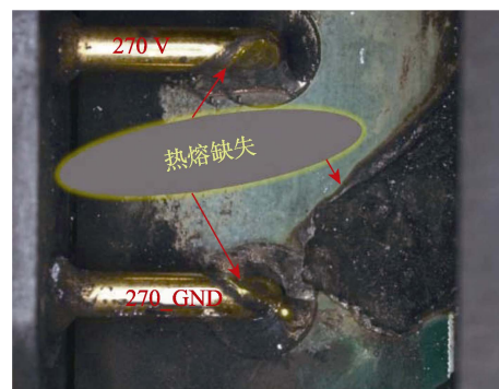
图 4 电源输入端引脚烧蚀形貌 Fig.4 Ablation morphology of the pins at the power input terminal
