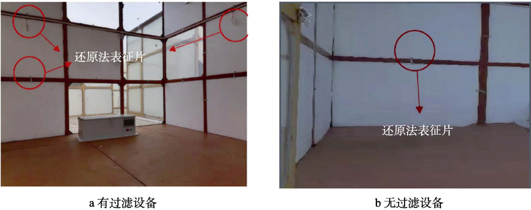
图 6 海南某试验棚下盐雾过滤效果验证实验 Fig.6 Verification test of salt spray filtration effect under a test shed in Hainan: a)with filtration equipment; b)withoutfiltration equipment
