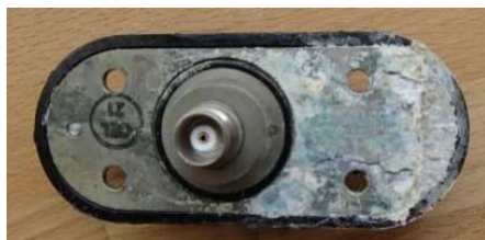
图2 天线连接结构腐蚀 Fig.2 Corrosion of antenna connection structure
