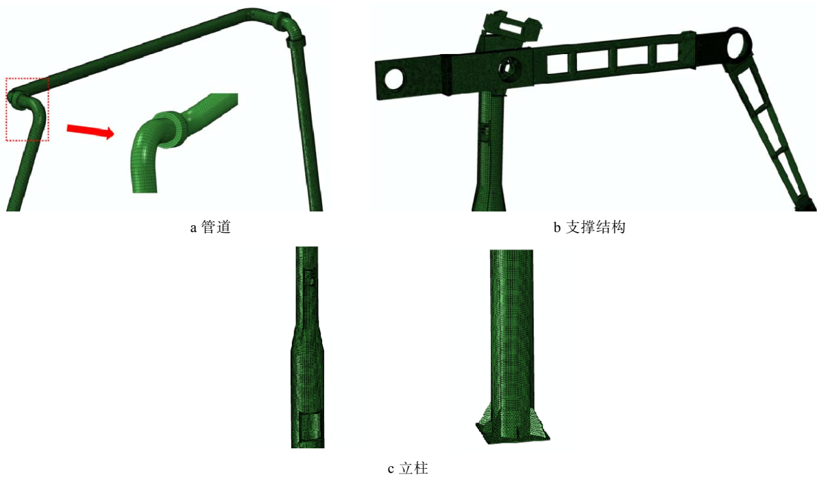
图 4 卸料臂整机结构网格划分 (局部) Fig.4 Meshing of complete unloading arm structure (local): a) pipe; b) support structure; c) column
