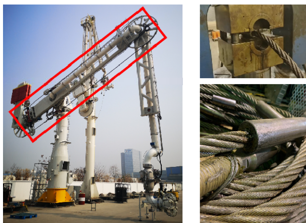
图 11 驱动钢丝绳缆安全系数的加强措施 Fig.11 Enhancement measures of drive wire cable safety factor
